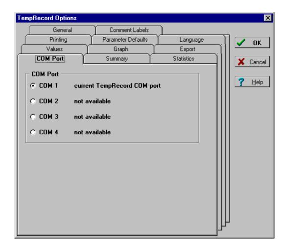
If your Reader Interface is connected to a COM port other than the one shown as Current **TEMPRECORD** Port, you will need to change the COM port setting. Click on the correct COM port number.
