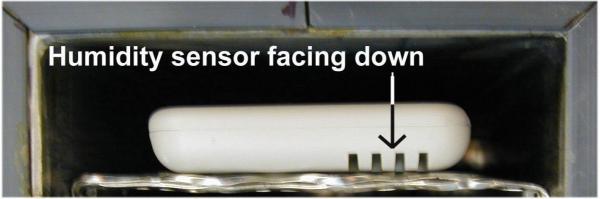
Drying the Humidity sensor in a **conventional oven** as recommended.
