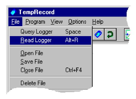
You will notice that some of the menu entries have keys alongside them, e.g. **File/Read Logger** has the key **Alt+R**. These keys are 'short-cut' keys that can be used to invoke that function. They are an alternative to opening the menus and selecting the function directly, in that they work from almost anywhere in the program.
